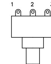
01 POTENTIOMETER PINOUTS - TOP VIEW
